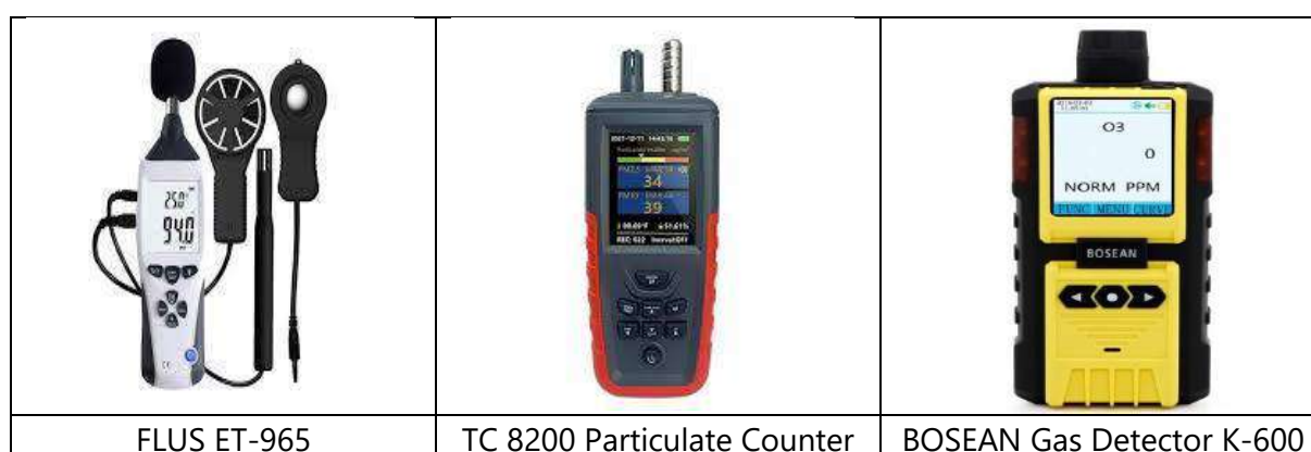
Figure 1: Noise level, dust and air quality measurement equipment
