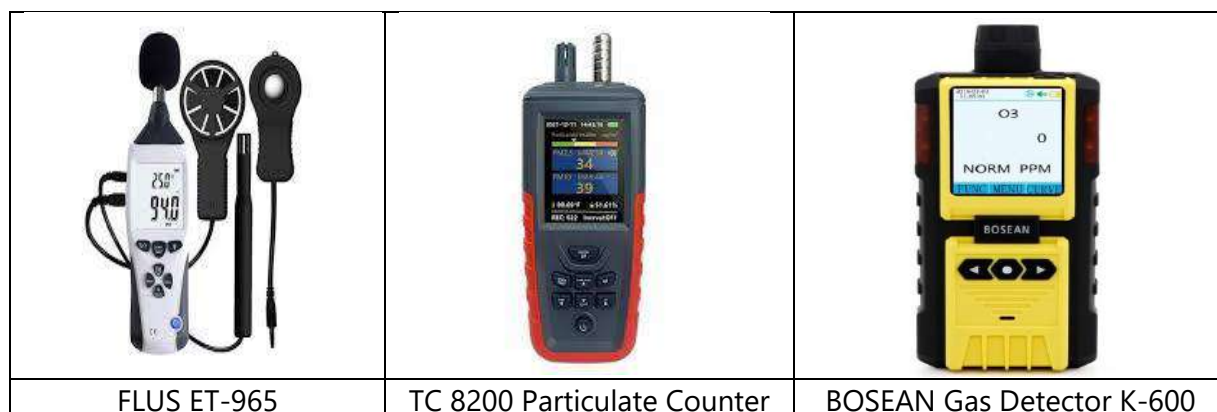
Figure 1: Noise level, dust and air quality measurement equipment
